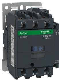
IEC contactor, TeSys D, nonreversing, 40A, 30HP at 480VAC, up to 100kA SCCR, 3 phase, 3 NO, 480VAC 60Hz coil, open style
