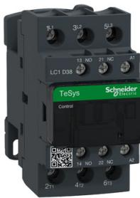
IEC contactor, TeSys Deca, nonreversing, 38A, 20HP at 480VAC, up to 100kA SCCR, 3 phase, 3 NO, 120VAC 50/60Hz coil, open
