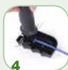
With one hand, hold the termination aid. With the other, press the handle completely down until the tool cycles impact.
