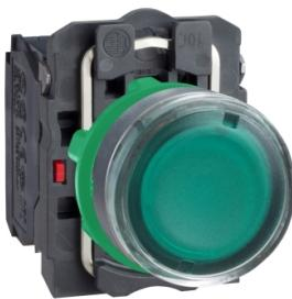
Illuminated push button, Harmony XB5, plastic, flush, green, 22mm, plain lens for BA9s bulb, spring return, lower than 250V, 1NO + 1NC
