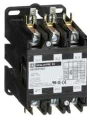
Contactor, Definite Purpose, 60A, 3 pole, 30HP at 575VAC, 3 phase, 110/120VAC 50/60Hz coil, open
