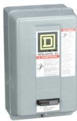
NEMA motor starter, Type S, nonreversing, Size 0, 18A, 2HP at 230VAC, 5kA SCCR, 1 phase, 2 pole, melting alloy, 120VAC coil, NEMA 1 [TAA]
