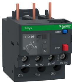
Thermal overload relay, TeSys Deca, 690VAC, 9 to 13A, 1NO+1NC, class 10A, for D12â€¢D38 unbalanced loads
