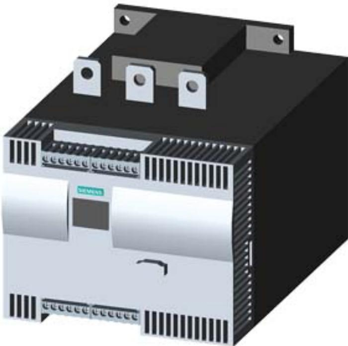
SIRIUS SOFT STARTER, VALUES WITH 460 V, 50 DEG., STANDARD: 280A, 200HP, INSIDE-DELTA CIRCUIT 3: 485A, 400HP, 200-460 V AC, 115 V AC, SCREW TERMINALS
