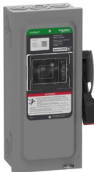
**Safety switch, heavy duty, fused, viewing window, NEMA 1, 240V, 30A, 3 pole, neutral installed**
