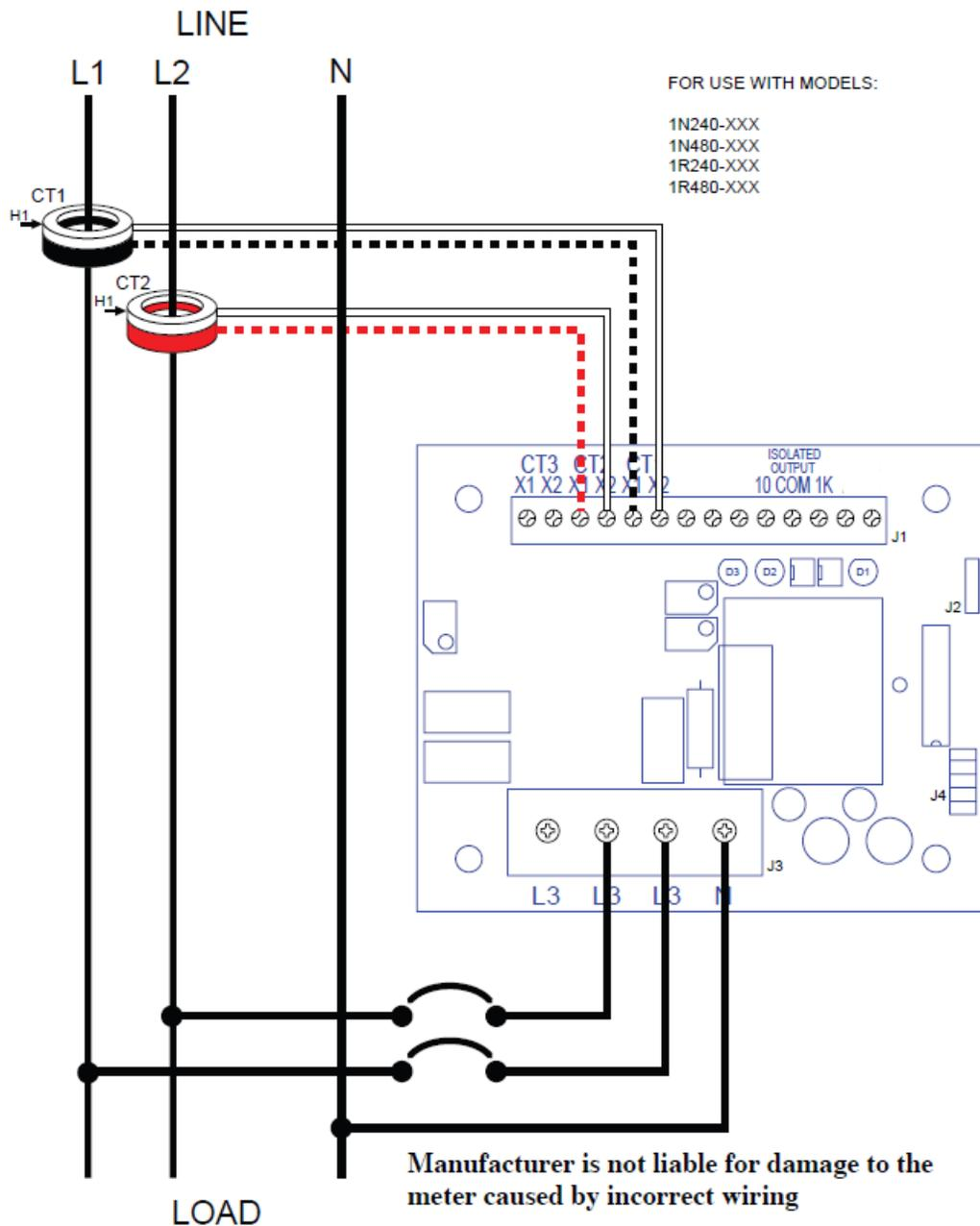
Figure 8: 1 or 2 phase, 3 wire Hookup Diagram
