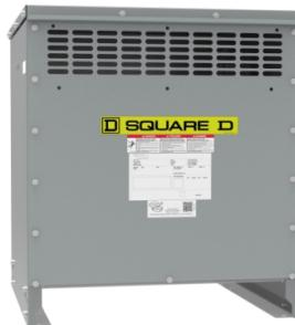
Transformer, dry type, DOE 2016, 30kVA, 3 phase, 240V delta primary, 480Y/277V secondary, 18M, 150C rise
