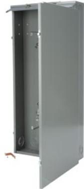
Siemens Energy Management Residential Specialty Load centers: 300-600 amp. Sub- Brand: Load Centers Type: 1: Application: Residential: Voltage Rating: 120/240V Amperage rating: 400A Phase: 1PH Load regulation: 400A Wiring configuration: 3w Bus Rating: 400 A Interrupt rating: 100000AIC. 400A ML 6 CKT LC 3R
