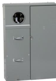
All in one, Homeline, CSED, ringed socket, 400A, semi flush mount, 30 spaces, 40 circuits, 25kA SCCR, no bypass
