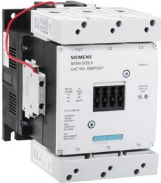
Non-reversing NEMA contactor, Size 6, Three phase full voltage, Contactor amp rating 540A, 3 wire (NO aux included), 440-480V 50-60Hz/DC coil, Non-combination type, Enclosure NEMA type (open), No enclosure
