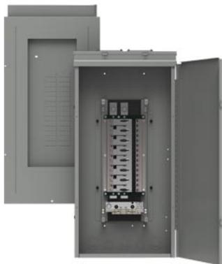
Siemens Low Voltage Residential Specialty Load centers: 300-600 amp. Load Centers Type: 1 Application: Residential V. Rating: 120/240V A. Rating: 400A Phase: 1PH Load regulation: 400 A Wiring conf.: 3w Bus Rating: 400 A Interrupt rating: 100000AIC No. of spaces: 30S Size (H x W x D): 9047.556 Mounting: Surface Enclosure: Outdoor NEMA 3R
