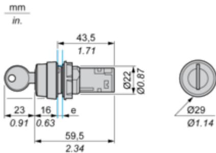
e Support panel thickness: 1 to 6 mm/0.4 to 0.24 in. (metal), 2 to 6 mm/0.8 to 0.24 in. (plastic).
