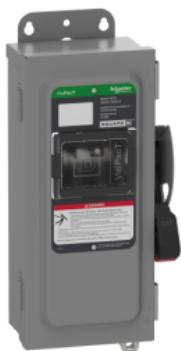
**Safety switch, heavy duty, fused, viewing window, NEMA 12, 240V, 30A, 2 pole, ground lugs**
