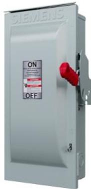
Siemens Low Voltage Circuit Protection Heavy Duty Safety Switch. 3-Pole 3-Fuse and solid neutral Fused in a type 3R enclosure (outdoor). Rated 600VAC (100A).
