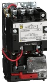
NEMA motor starter, Type S, nonreversing, Size 0, 18A, 5HP at 460VAC, up to 100kA SCCR, 3 phase, 3 pole, Motor Logic, 120VAC coil, open [TAA]
