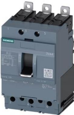
circuit breaker 3VA4 UL frame 125 breaking capacity class M 35kA @ 480 V 3-pole, line protection TM210, FTFM, In=60A overload protection Ir=60A fixed short-circuit protection Ii=10 x In clamp connection
