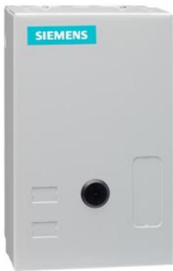
Electrically held lighting contactor, Contactor amp rating 30A, 0 N.C. / 4 N.O. Poles, 110VAC 50HZ/120VAC 60HZ coil, Non-combination type, (no disconnect device), Enclosure NEMA type 1, Indoor general purpose use
