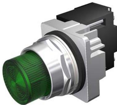
30mm Command/52, Chrome Finish Heavy Duty, Watertight/Oiltight Complete Metal Unit Illuminated Indicator Light Full Voltage type, 120V AC/DC LED Lamp, BA9s Plastic Lens, Green UL Listed, CSA Certified NEMA 1,3,3R,4,4X,12,13 & Automotive Standards
