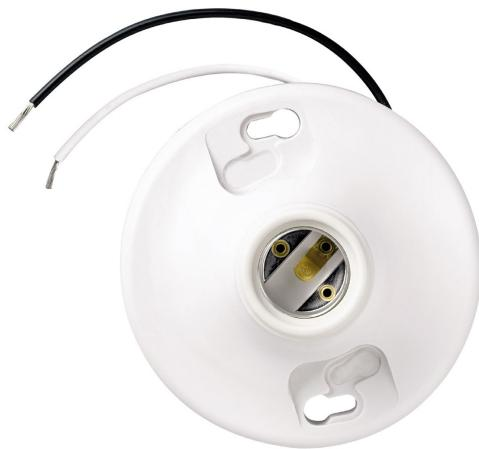
Medium base, phenolic, one-piece keyless, 4 terminals with Tamper-Resistant-drive screws, fits 3 1/4-inch and 4-inch boxes, with cage necks, 6-inch Leads.
