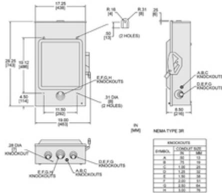
WHEN MOUNTING THESE SWITCHES, ALLOW 4.50 [114] MM CLEARANCE
