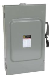
Safety switch, general duty, non fusible, 3 pole, 3 wire, 240VAC, 200A, Type 3R with bolt on hub prov
