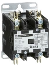
Contactor, Definite Purpose, 30A, 2 pole, 5HP at 230VAC, 1 phase, 110/120VAC coil at 50/60Hz, open
