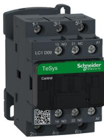
IEC contactor, TeSys Deca, nonreversing, 9A, 5HP at 480VAC, up to 100kA SCCR, 3 phase, 3 NO, 230VAC 50/60Hz coil, open style
