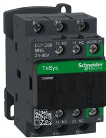
IEC contactor, TeSys Deca, nonreversing, 9A, 5HP at 480VAC, up to 100kA SCCR, 3 phase, 3 NO, 24/60 VAC/VDC coil, open
