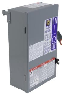
Plug-in unit, I-Line Busway, fusible, 200A, 240VAC, 3 pole, 3 fuse + G, plug in connection
