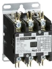
Contactor, Definite Purpose, 30A, 3 pole, 20HP at 575VAC, 3 phase, 110/120VAC 50/60Hz coil, open
