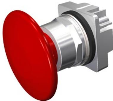
30mm Command/52, Chrome Finish Heavy Duty, Watertight/Oiltight Metal Operator, Round Push-Pull Operator Non-illuminated Mushroom Head Cap Large 2 1/2" (63.5 mm) Plastic, Red 2 Position Maintained, Pull-to-Release UL Listed, CSA Certified NEMA 1,3,3R,4,4X,12,13 & Automotive Standards
