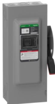
**Safety switch, heavy duty, fused, viewing window, Type 1, 240V, 100A, 3 pole, neutral installed**
