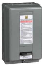
Starter, Definite Purpose, nonreversing, 30A, 2 pole, 1 phase, 208V to 240V AC coil, melting alloy overload, NEMA 1
