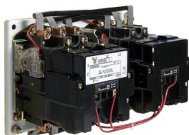
NEMA Contactor, Type S, reversing, horizontal, Size 3, 90A, 50HP at 575VAC, 3 phase, up to 100kA, 3 pole, 120VAC coil, open style [TAA]
