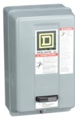
NEMA motor starter, Type S, nonreversing, Size 1, 27A, 10HP at 460VAC, 5kA SCCR, 3 phase, 3 pole, melting alloy, 208VAC coil, NEMA 1 [TAA]
