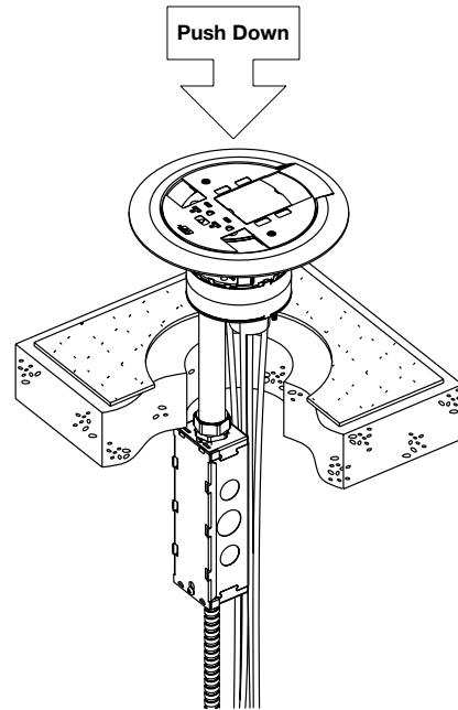
**CAUTION:** Poke-Thru cannot be rotated in hole after inserted into floor.
