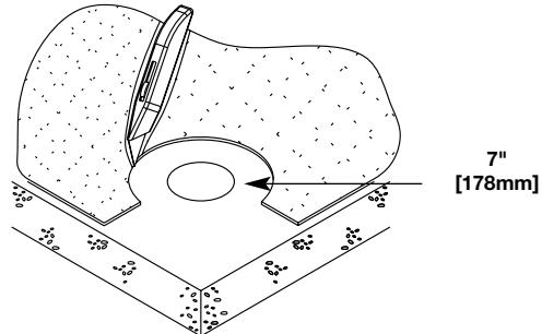
**CAUTION:** For tile installations up to a maximum of 3/4" [19.1mm] thick.
