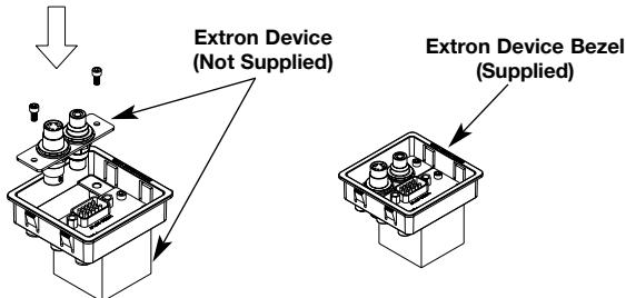
**NOTE:** This Bezel Accommodates (1) Single and (1) Double or (3) Single MAAPs (Mini Architectural Adapter Plates) Extron Devices.
