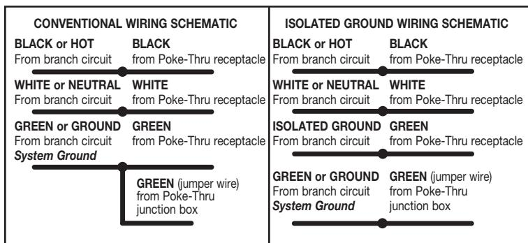
**WARNING:** Ground wire from junction box must be connected to system ground.
