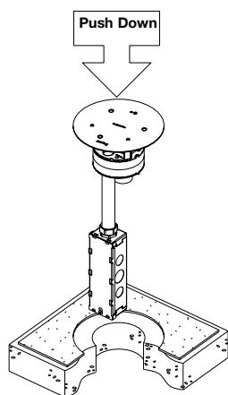
**CAUTION:** Poke-Thru cannot be rotated in hole after insertion into floor.
