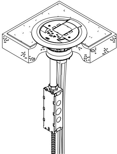
**Step 13** Push Poke-Thru unit into concrete to complete installation.
