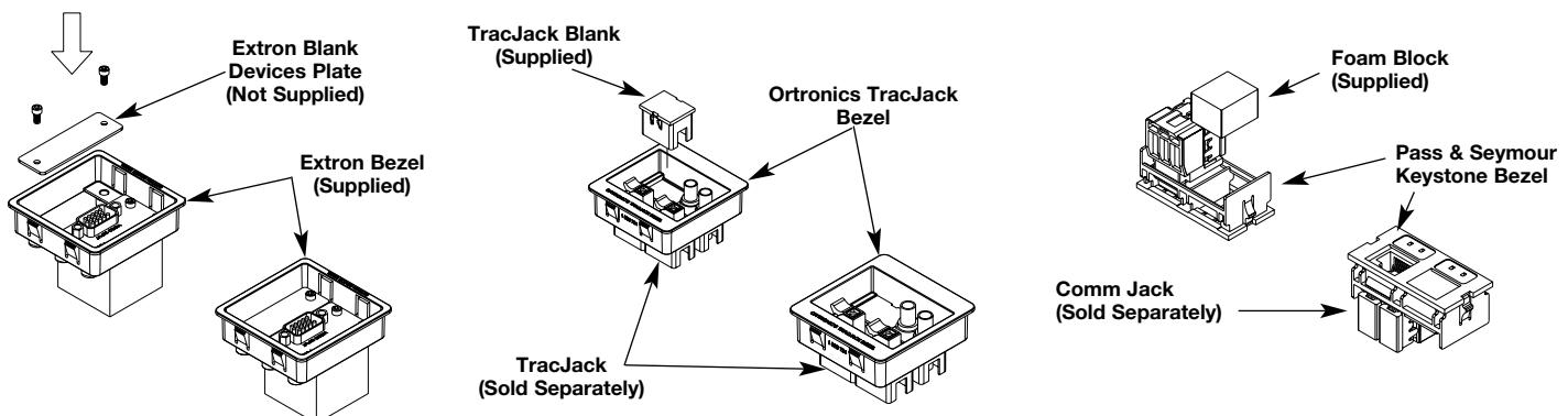
**CAUTION: Empty communication ports must be closed off with foam blocks, TracJack blanks or Extron Single and/or Double MAAP blanks to maintain Fire Classification.**
