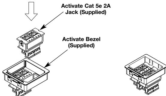
**Pass & Seymour ACTIVATE Bezel and Communication Jack (Supplied with AV3ATC & AV3CTC units).**
