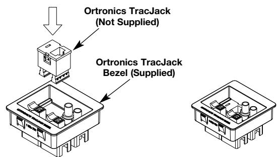
**Ortronics TracJack Bezel & Communication Jack (Bezel Supplied with AV3ARTTC and AV3CRTTC, TracJacks sold separately).**
