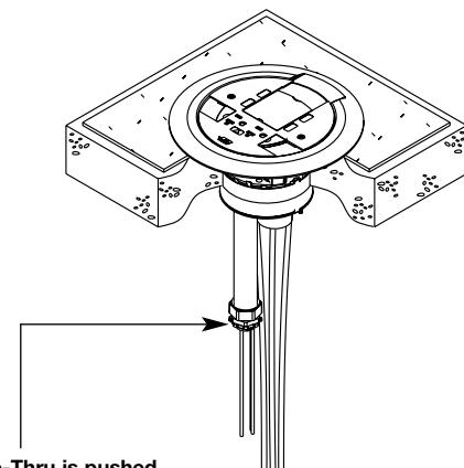
Once Poke-Thru is pushed into the Cored Hole, from below, install an EMT Compression Fitting (Not Supplied) and Junction Box (Not Supplied) to the Conduit System. Complete installation per NEC and Local Codes.
