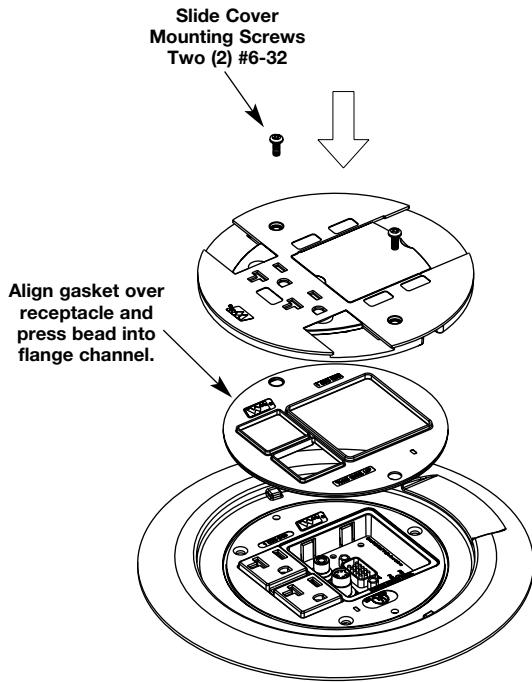
**CAUTION:** Gasket must be set in place to provide scrub water seal.
