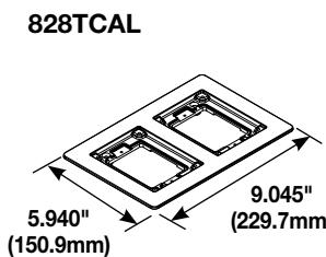
**Two-Gang Brushed Aluminum Combination Carpet and Tile Flange** – Accepts Ortronics® MAB6TJ TracJack and MAB3S2 Series II adapters and Wiremold CM Series inserts, sold separately.
