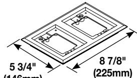
**Two-Gang Nonmetallic Carpet Flange** – Available in black or brown. For Ortronics® connectivity use with 829PFLRT Cover. For Activate connectivity use with 829PFL Cover. Accepts Ortronics® MAB6TJ TracJack and MAB3S2 Series II adapters and Wiremold CM Series inserts, sold separately.
