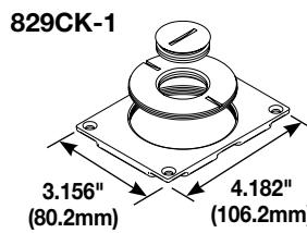
**Brass Communication Cover Plate** – 2 5/8" and 1" (67mm and 25mm) plugs.
