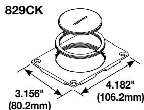
**Brass Communication Cover Plate** – 2 5/8" and 2 1/4" (67mm and 57mm) plugs.
