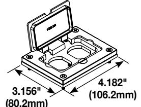
**Brass Rectangular Cover Plate** – Allows for mounting of a duplex style receptacle with a rectangular style flip lid cover.
