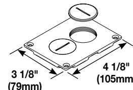
**Brass Duplex Cover Plate** – Screw plugs. Screw plugs are 1 1/2" (38mm) in diameter.
