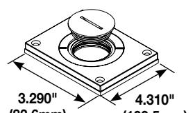
**Brushed Aluminum Cover Plate** – Power or communication plate with 2" (51mm) and 1 1/4" (32mm) plugs.
