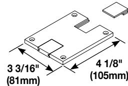
**Nonmetallic Communication Cover Plate** – Data slides. Available in black or brown. Feed through only, not for use with a mounting plate for communication jacks.
