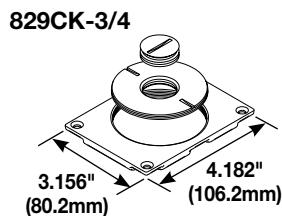
**Brass Communication Cover Plate** – 2 5/8" and 3/4" (67mm and 19.1mm) plugs.
