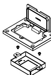
**A/V Adapter Plate** – Sheet metal adapter plate that accepts two (2) Extron® Electronics MAAP style device plates (sold separately). For use with 828GFITC, 828GFITCAL or 828PRGFI cover plates. (Sold separately.)
