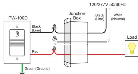
Wiring for PW-101D with a neutral connection.
