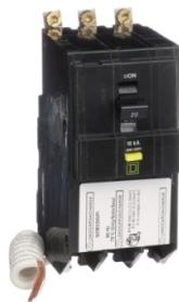
Mini circuit breaker, QO, 20A, 3 pole, 208Y/120VAC, 10kA, bolt on, 6mA grd fault A, pigtail [TAA]
