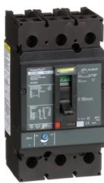
Circuit breaker, PowerPact J, 225A, 3 pole, 600VAC, 14kA, lugs, thermal magnetic, 80%
