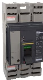
Circuit breaker, PowerPact P, 1200A, 3 pole, 600VAC, 25kA, lugs, Micrologic 5.0, 80%
