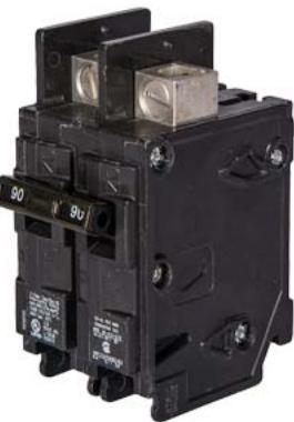
Siemens Low Voltage Molded Case Circuit Breakers General Purpose MCCBs - Type BQ, 2-Pole, 120/240VAC are Circuit Protection Molded Case Circuit Breakers. 2-Pole Common-Trip circuit breaker type BQ. Rated 120/240V (125 A) (AIR 10 kA). Special features: line side lugs included. Note: Load side lugs are included.
