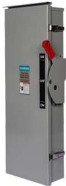
Siemens Low Voltage Circuit Protection Heavy Duty Safety Switches. Type: ENCLOSED, SAFETY SWITCH Std: UL V. Rating: 600V A. Rating: 60A Wattage: 3W No. Of Poles: 3P F. Rating: 60Hz Action: DOUBLE THROW Material: STEEL Enclosure: TYPE 1. 2-3 point mounting holes. O. Cycles: 10000 O. Temperature: (-20F-120F) AMBIENT TEMPERATURE Environmental Conditions: INDOOR
