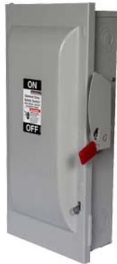
Siemens Low Voltage Circuit Protection General Duty Safety Switch. 2-Pole or 3-Pole Non-Fused in a type 1 enclosure (indoor). Rated 240VAC (100A). Horse power: 1-PH 2-W (15), 3-PH 3-W (30), 250VDC (20). Special features: service entrance labeled suitable for 3-PH motor loads.
