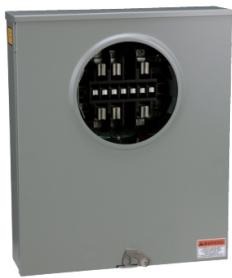
Meter socket, ringless, 3 phase, 4 wire, 20A, 13 jaws, 600VAC max, solid top, no bypass, no jaw release
