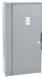
**Safety switch, heavy duty, fusible, 800A, 4 wire, 3 pole, 1 neutral, 500hp, 600VAC/DC, NEMA 3R**
