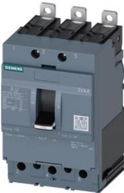
circuit breaker 3VA4 UL frame 125 breaking capacity class S 25kA @ 480 V 3-pole, line protection TM210, FTFM, In=15A overload protection Ir=15A fixed short-circuit protection Ii=20 x In clamp connection
