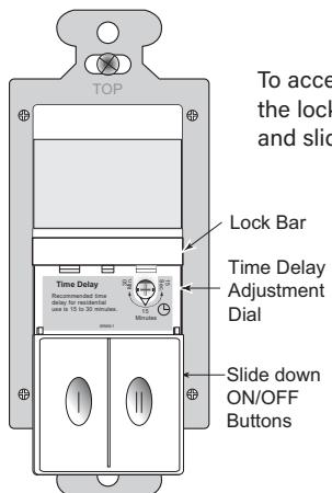
To access adjustment dial, gently pull the lock bar away from the switch face and slide the on/off buttons down.
