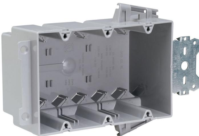
Triple Gang, Wood and Steel Stud Bracket Box with Quick/Click. 3/8-inch offset for wood and steel stud mounting. Six Auto/Clamps on each end. For use with 3/8-inch to 5/8-inch wallboard.
