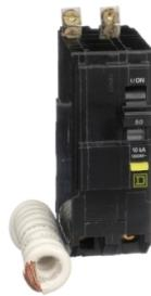
Mini circuit breaker, QO, 50A, 2 pole, 120/240VAC, 10kA, bolt on, 6mA grd fault A, pigtail [TAA]
