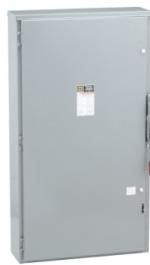
**Safety switch, heavy duty, fusible, 400A, 4 wire, 3 pole, 1 neutral, 250hp, 600VAC/DC, NEMA 3R**
